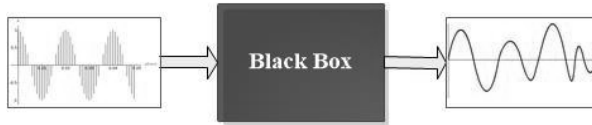
Fig. 2. An input is applied to the system, and it is observed how the output is affected.
